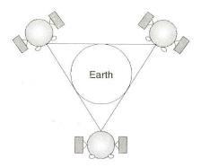
Fig.2.21 Three Satellites to Cover the Planet
