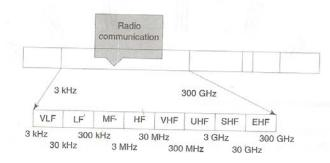
Fig 2.18. Radio Communications Band
