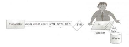
**Fig. 2.38** Discarding Non-SYN Characters Until SYN is Received for Synchronization When the clock starts measuring the bit values, the counter within a receiver is increment every bit receive and Measured and pushed into the character assembler within the receiver. This is as shown in Fig. 2.39.
