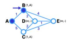
In this step, like in step 2, the status record set of tentative nodes that have a direct link to T-node (D, E), has been changed. Also, MCA-301 244 since D has less weight, it has been chosen as T-node and its label has changed to permanent (see below).
