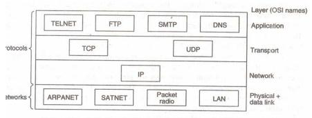
Figure 1-22. Protocols and networks in the TCP/IP model initially.
