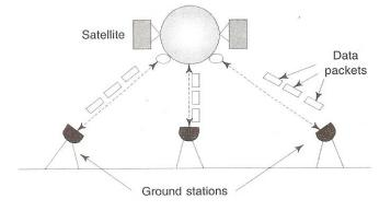
Fig.2.23 Time Division Multiple Access (TDMA)
