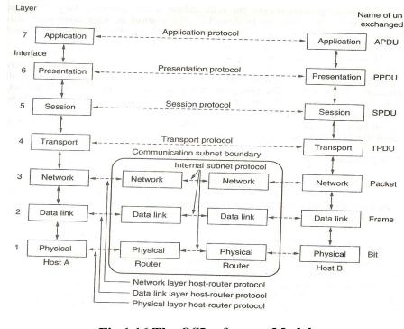
Fig 1.16 The OSI reference Model
