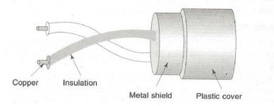
Fig 2.11. Shielded Twisted Pair (STP)
