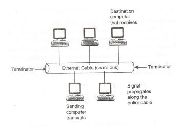
Fig 1.3 Signal flow across an Ethernet
