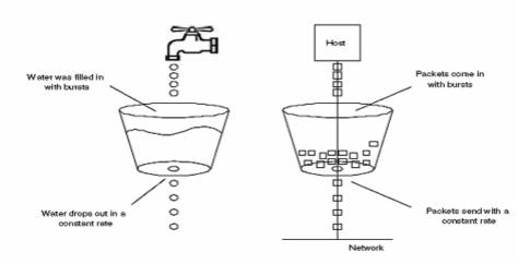
Figure 6.6: Leaky Bucket Algorithm
