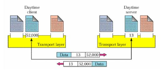
Figure 7.8: Addressing at Transport Layer
