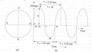
Fig. 2.4 Sinusoidal Signal
