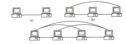
Figure 1.9 (a), (b), (c) Number of connections for 2,3,4 computers, respectively
