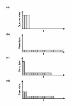
Figure 6.7: Traffic Shaping with Leaky and Token Bucket Algorithms
