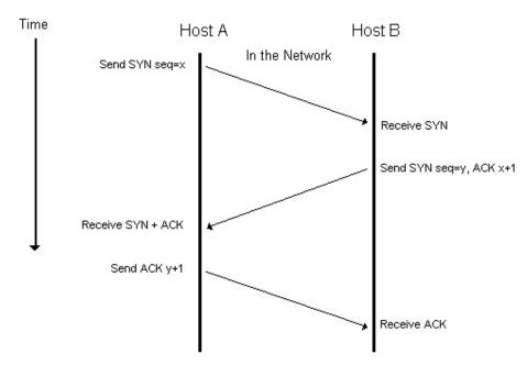
Figure 7.15 - TCP Connection Establishment
