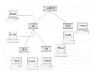
The central hub contains a repeater, which looks at the incoming bits and regenerates them afresh as the full blown signals for 0 or 1 as required. This allows the digital signals to traverse over longer distances. Therefore, the
