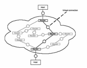
Figure 6.9: Admission control in computer networks
