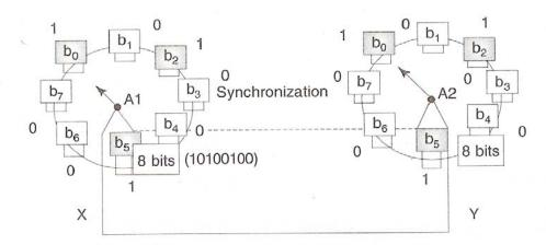
Fig 2.34. Serial Transmission and Synchronization
