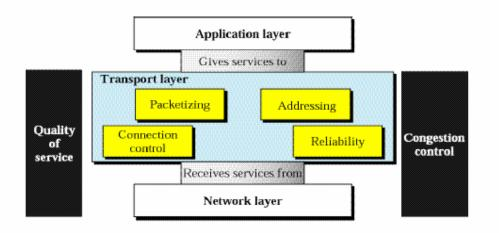
Figure 7.1: Transport Layer in ISO-OSI Reference Model
