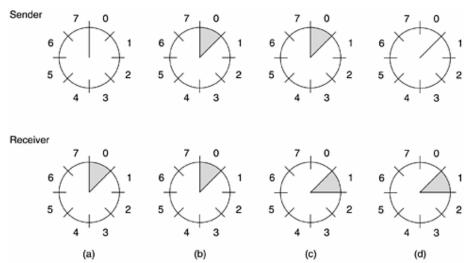
given the next highest sequence number, and the upper edge of the window is advanced by one. When an acknowledgement comes in, one advances the lower edge. In this way the window continuously maintains a list of unacknowledged frames. Figure 5.4 shows an example of 8-windows.
