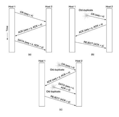
Figure 7.5: Three protocol scenarios for establishing a connection using a three-way handshake. CR denotes CONNECTION REQUEST. (a) Normal operation. (b) Old duplicate CONNECTION REQUEST appearing out of nowhere. (c) Duplicate CONNECTION REQUEST and duplicate ACK.
