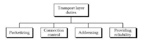
Figure 7.6: Functions / Duties of Transport Layer
