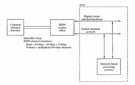
FIGURE 8.4: Block diagram of ISDN functions.
