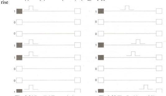
Fig. 2.31 Parallel Transmission
