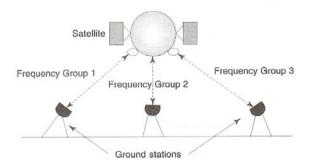
Fig.2.22 Frequency Division Multiple Access (FDMA)
