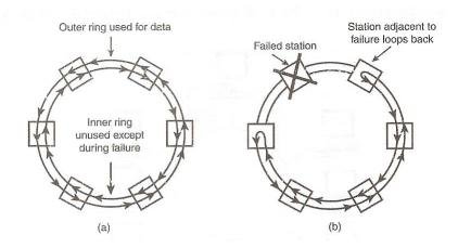
Figure 1.5 (a) FDDI network with counter ring (b) the same network after a station has failed
