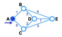
In this step, you see that the status record set of tentative nodes directly linked to T-node (B, C) has been changed. Also, since B has less weight, it has been chosen as T-node and its label has changed to permanent (see below).
