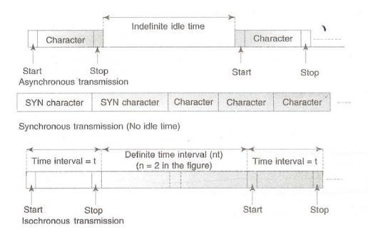
Fig.2.40 Asynchronous, Synchronous and Isochronous Transmissions
