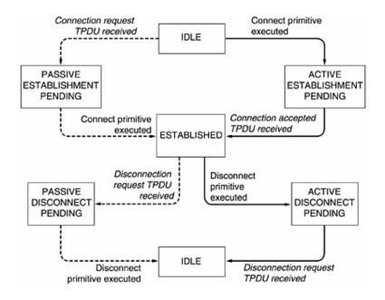
Figure 7.4: State diagram of Connection establishment & release.
