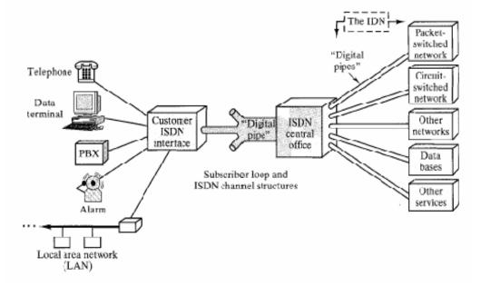
Figure 8.3: Conceptual view of ISDN connections
