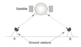
Fig.2.20 Satellite Microwave Communication
